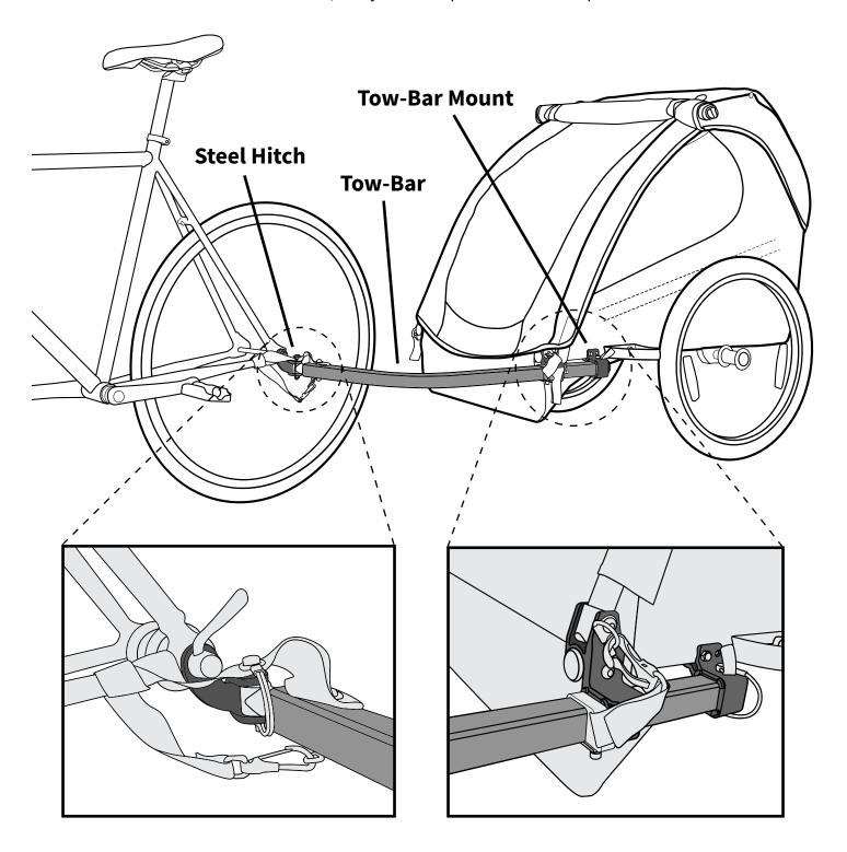
Every Burley trailer comes equipped with a Steel Hitch, Tow-Bar and Tow-Bar Mount. In most cases this is all you will need to safely connect the trailer to your bicycle. In some cases you may require an additional adapter or thru-axle. This guide will help you determine if you require one of these additional parts, and if so, which part you require.
